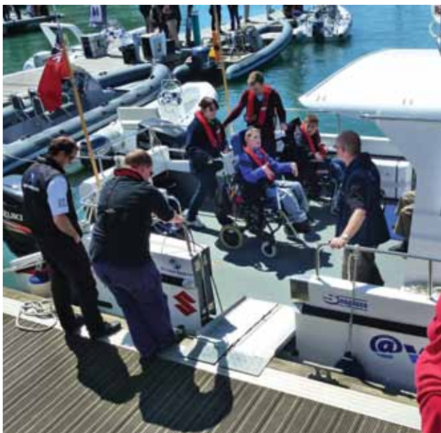
Side doors can provide access points if wide enough
